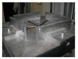
Figure 2: Support for EN14488-5 test
