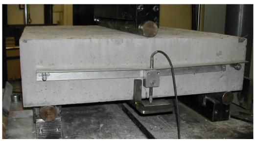
Figure 6: 3-point bending test on square panels cast in situ test set-up
