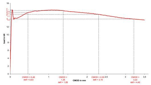
Figure 7 - Load-displacement curve of a 3-point bending test on square panels
