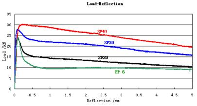
Figure 9: Comparison of Load-Deflection curves of FRC panels with different fibres. Each plot represents the mean result for each set of nine panels.[7]
