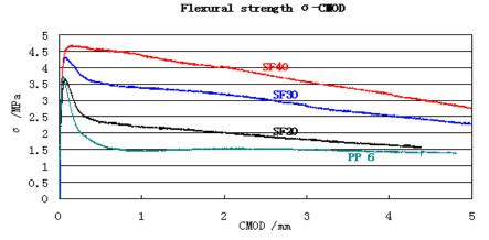
Figure 10: Comparison of flexural strength in the FRC compared to CMOD.[7]
